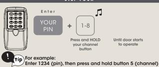
Pressing the channel button (1-8) again within 10 seconds will control the garage door again.
